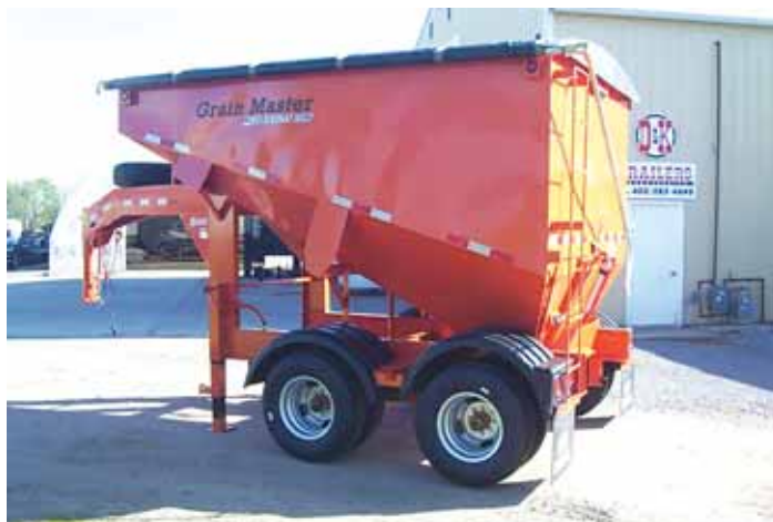
Gradual 30-degree rearward slope ensures easy unloading of grain and mixed or pelleted feeds.
