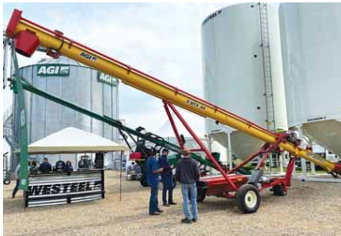
Auger makes it possible to unload a truck remotely from the cab or to control it directly using an exterior joystick.
