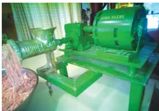
"I removed the hand crank and fabricated a drive shaft from old steel nuts," Froemming says.
