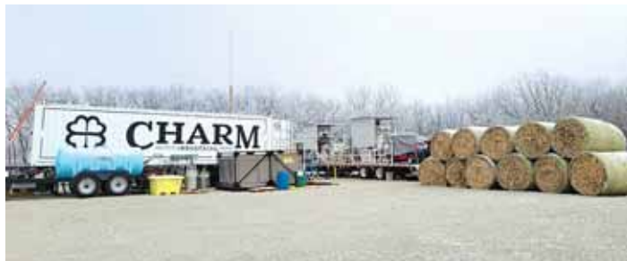
ISU bio-oil crop residue-production site. Sites can process up to 10 tons of feedstock per day.
