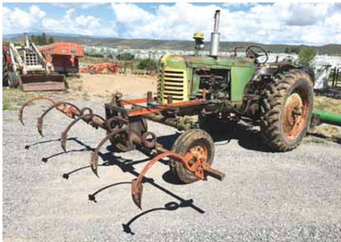
“The spades are set so I can drive up to the gated pipe, drop them down, and drag the furrows straight back to meet the ones in the field,” says Krush.
