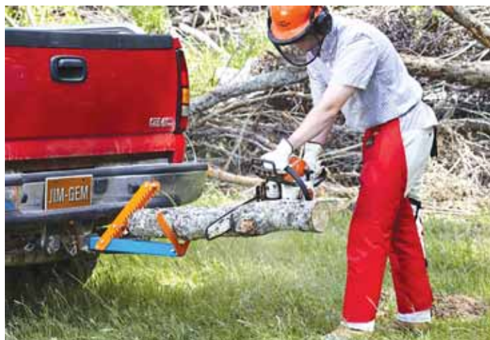
Jaw Boss can handle branches or small logs, as well as dimension lumber ranging from 2 to 9 in. in diameter.
