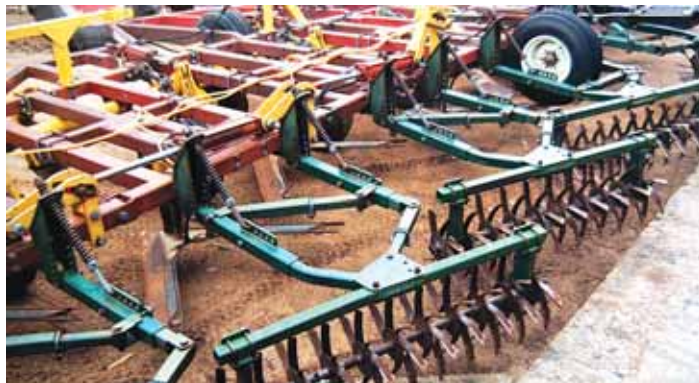
To get the most out of tillage equipment, Kuntz's mantra is go fast, go shallow, go home. To do so, he emphasizes not only leveling but also removing attachments from the rear of the implement.
