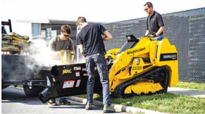
Mini MAC is a compact mixing and conveying bucket engineered for mini tracks and skid loaders.
