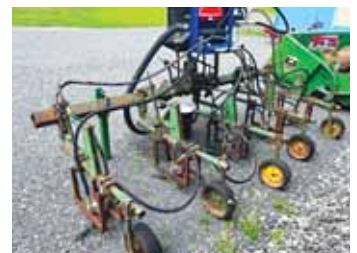
“We’re using an R-Tech IRM-X4 in our experiments. This multi-row, tractor-mounted inter-row mower has a hydraulic motor that spins four swing blades, attached to a central disk, at 1,800 rpm.”
