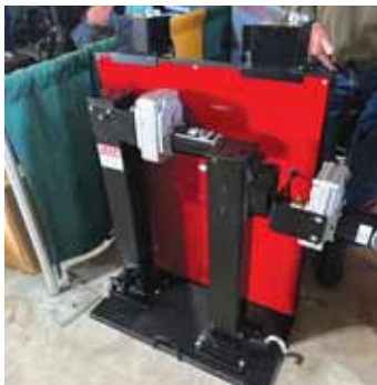
"They'll fit any 4-in. manual trailer jack on the market. The kits are rated at 12,000 lbs.," says Walters.
