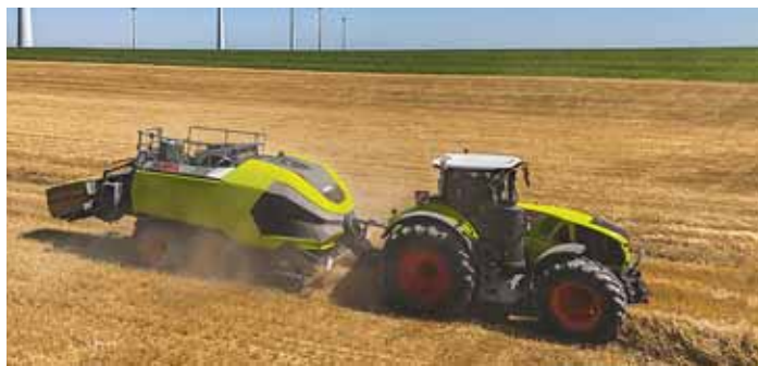
Futuristic Claas baler will feature advanced sensors that continuously monitor gear loads, enabling AI-assisted systems to adjust press density and bale length in real time.
