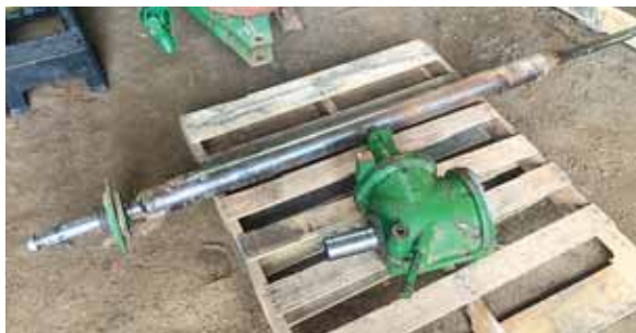
Countershaft and gearbox pulled from combine.
