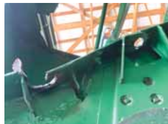
Bracket after countershaft failed.
