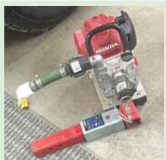
Water pump and 2 by 2-in. receiver hitch insert.
